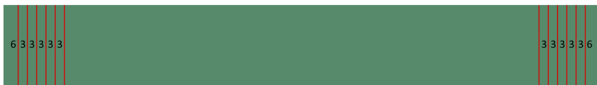
Figure 9 – Gunnel Cut Plan – Top Surface of Panel
